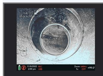
The Hathorn Info Bar at the bottom of the screen allows you to see battery life, speaker function, time and date, recording file location, zoom, sonde frequency/function and footage. The info bar is customizable - allowing you to put your company or client info at the bottom of the screen, recorded throughout the video. The newly designed, intuitive menus allow for a minimal learning curve. You are up and running in minutes.
